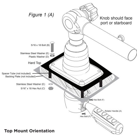
Mount orientation on top with locking pin facing outboard
